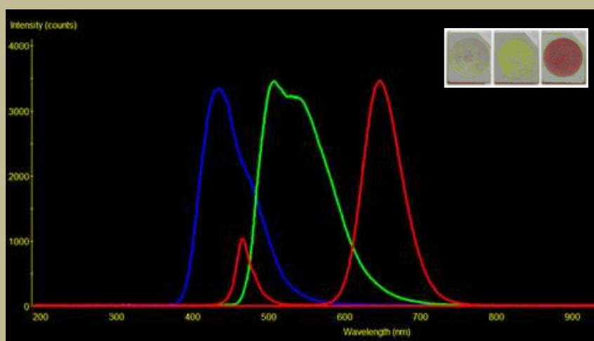
The entire 400 nm to 700 nm visible region is covered by the three LEDs (the small peak in red colour is a weak secondary emission from Spectrafill red LEDs). White light synthesised by combining the light from three separate Spectrafill devices has a significantly flat spectral distribution – ideal for
