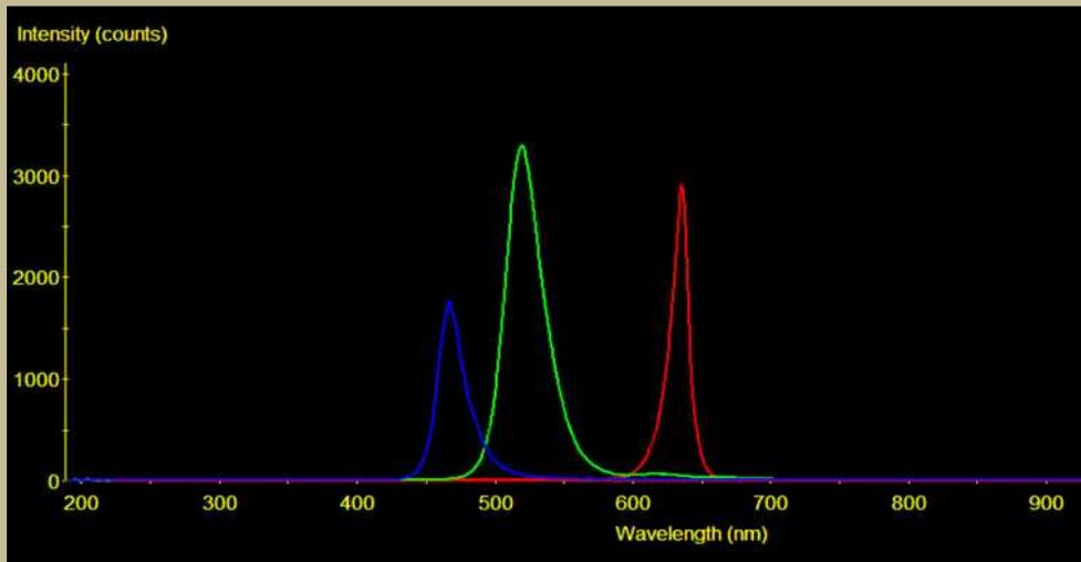
Thanks to the nearly flat white spectrum that results from mixing light from Spectrafill RGB LEDs, the lighting quality is much improved from what can be obtained with single white LEDs. This is, therefore, a much superior way of creating high-quality white light. Fixed drive systems can be implemented with Spectrafill LEDs to generate light with a fixed spectral distribution. With a little more sophistication, full spectral variability can also be implemented.
