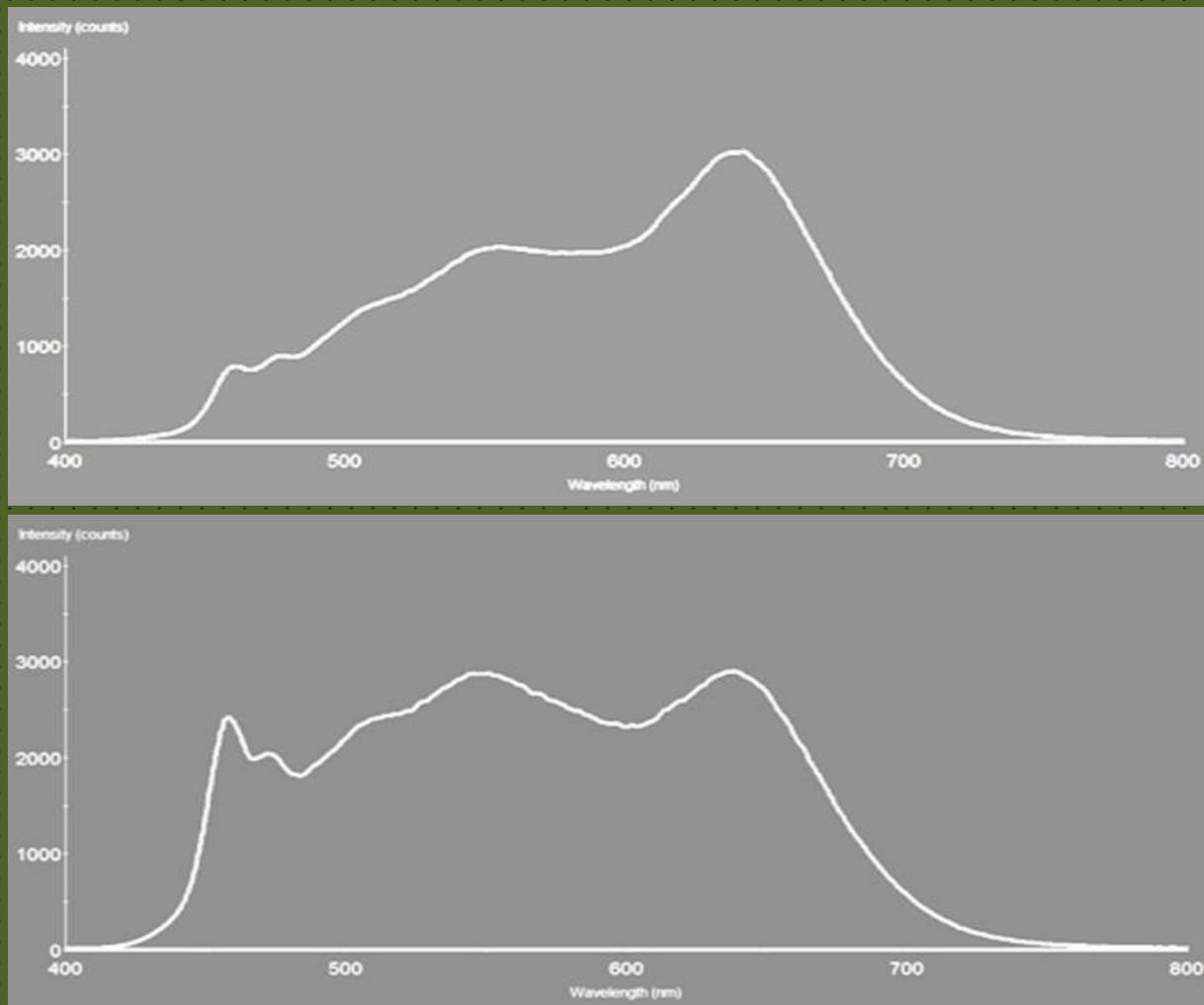
Tungsten LEDs have a nominal colour temperature of 4315 Kelvin whereas the flat-white LEDs have a nominal colour temperature of 6162 Kelvin.
